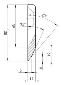
Blade sharpening wear limit 80mm to 60mm **Figure 11**
