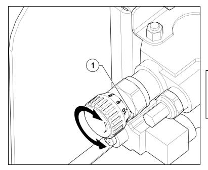
1 CONTROL VALVE FEED SPEED ADJUSTMENT.
