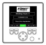
Turn ignition key fully clockwise to crank engine. Display will automatically go to P1
