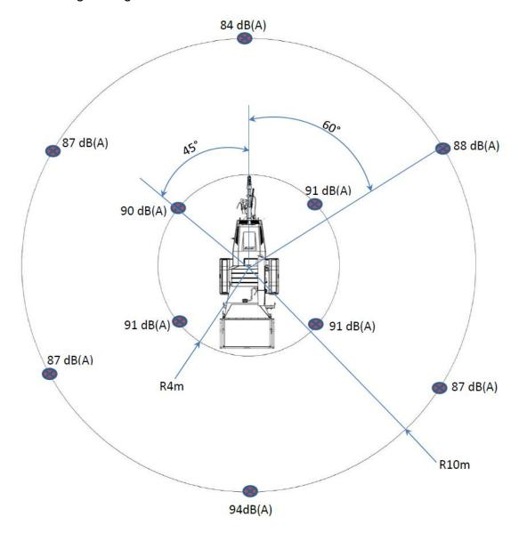
A-weighted emission sound pressure (beside operator's ear) LpA = 106.3dB(A). Peak C-weighted instantaneous sound pressure (beside operator's ear) LCpeak = 128.4dB(C). Results at 10 metre radius are calculated.
